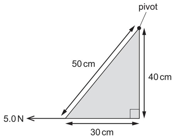
A cord is attached to the bottom left corner of the sheet and pulled with a horizontal force of 5.0 N to the left.
